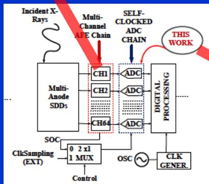
Asynchronous Noise-Shaping SAR ADC
