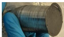
Figure: Initial condition of the sample vessel head, undermark the black oxide film development on the stainless steel layer.
