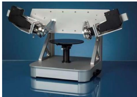
Semilab inSE-1000 in-situ ellipsometer
