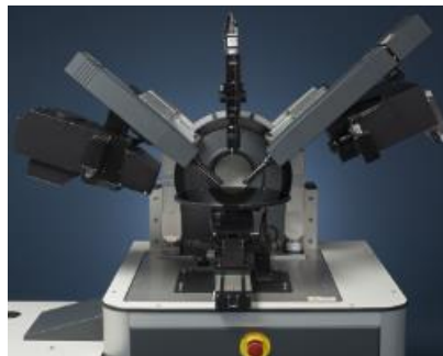
Semilab SE-2000 ex-situ ellipsometer
