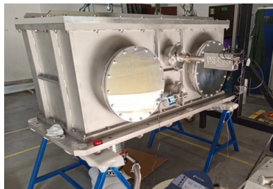
EA1 Double Turning Chamber nearing completion
