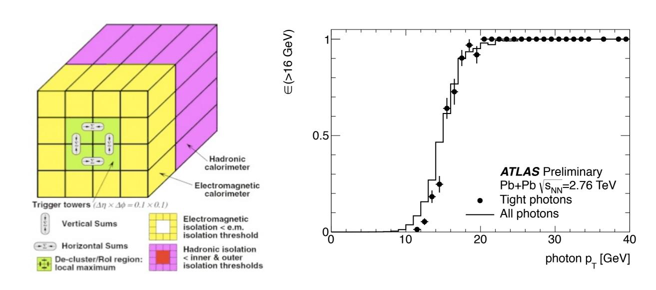
Use ATLAS electromagnetic object trigger, based on combinations of 0.1x0.1 "towers" and threshold of 16 GeV: 0.2x0.2 sliding window but trigger is only on 0.2x0.1 regions
