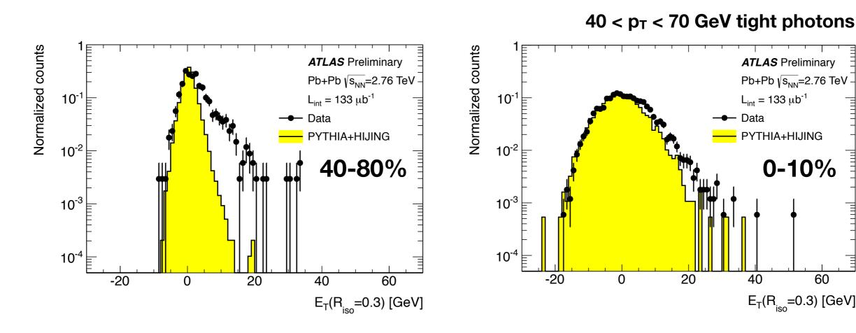
Sum of transverse energy within R=0.3 cone EM energy in 5x7 cells removed to remove photon
