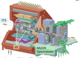
Centrality selection based on a geometrical Glauber model fit of the V0 scintillators amplitude
