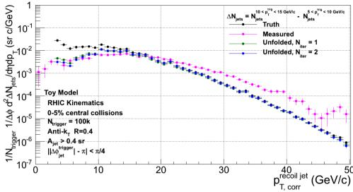
Unfolding converges stably to Truth above  $p_{\scriptscriptstyle T}^{\scriptscriptstyle trigger}$  threshold
