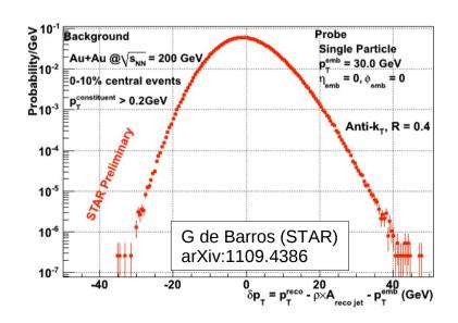
Crucial feature for unbiased measurement:  $\delta p_T$  distribution is independent of fragmentation pattern of embedded jet (G de Barros (STAR) arXiv:1109.4386)
