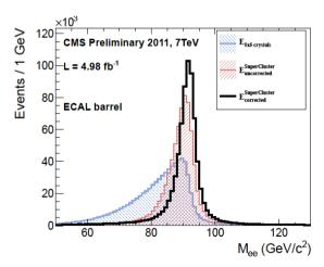
These two plots show the impact on the Z→ee energy scale and resolution from the incorporation of more sophisticated clustering and cluster correction algorithms.
