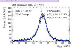
Invariant mass distribution of  $Z \rightarrow \mu\mu\gamma$  final states from 2011 DATA. The photon energy scale and resolution are extracted from de-convoluting the Z line shape in this final state. Plots for DATA and MC for EB for R9>0.94, EB inclusive and EE inclusive.
