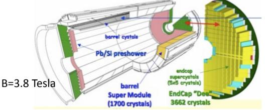
PbWO $_4$  Crystals  $\rho$  = 8.3.g/cm $^3$  61200 Xtals (25.8 X $_0$ ) in Barrel (EB)  $|\eta|$ <1.479) 14648 Xtals (24.7 X $_0$ ) in Endcaps (EE) 1.479< $|\eta|$ <3.0 Rad-Length X $_0$  = 0.89 cm Moliere radius r= 2.2 cm Light Yield Temperature dependence -2.2%/deg. Low light yield 4.5 pe/MeV on APD-pair or VPT but rapid light emission: 90 % in 25ns at 420 nm Transparency radiation dependant
