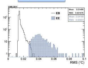
Temperature stability of the ECAL Barrel and Endcap detectors during the period April 2011 - October 2011.
