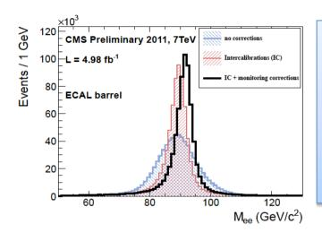
The top plot show the impact on the Z→ee energy scale and resolution that are obtained from applying energy scale corrections to account for the intrinsic spread in crystal and photo-detector response, and time-dependent corrections to compensate for crystal transparency loss.
