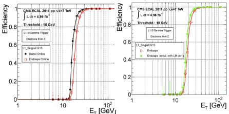
Trigger efficiency as a function of ET for an trigger path with a threshold of 15 GeV for the barrel and the endcap.
