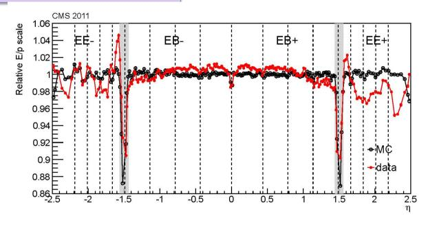
Relative energy scale as measured from the energy-momentum balance in W $\rightarrow$ ev decays as a function of pseudo rapidity  $\eta$ . The measured scale shows a much larger variation as a function of  $\eta$  than the MC. The scale is DATA is adjusted to the one observed in MC
