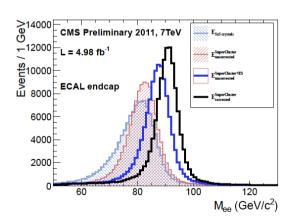
Good energy resolution is achieved with preliminary energy calibration for 2011. Instrumental resolution (obtained from Z -> ee invariant mass with ECAL energies and electron track directions): 1.0 GeV in ECAL Barrel
