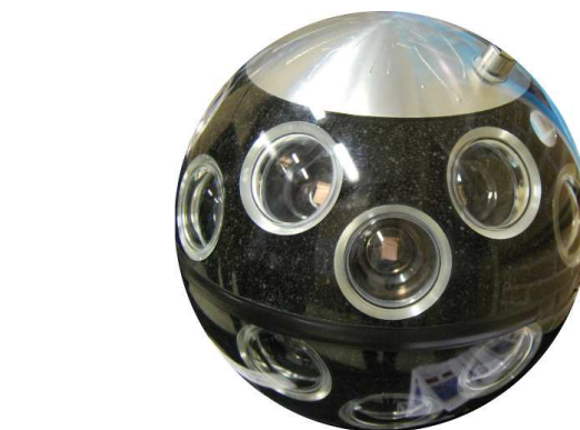
Figure 1: A mechanical reference model of a multi-PMT OM showing various PMTs, surrounded by an expansion cone, in a 17-inch diameter glass sphere.
