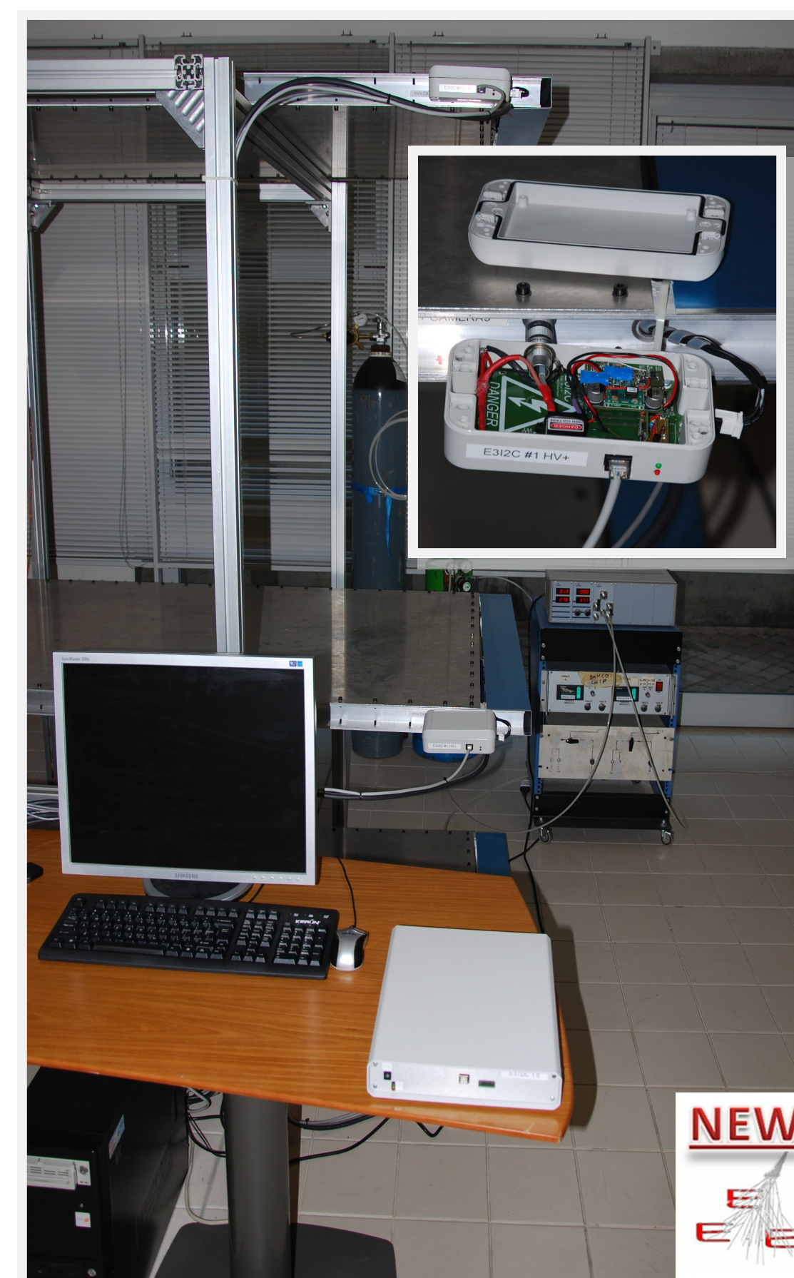
An MRPC of the EEE telescope equipped with 2 NINO boards and 2 E 3 I 2 C boxes
