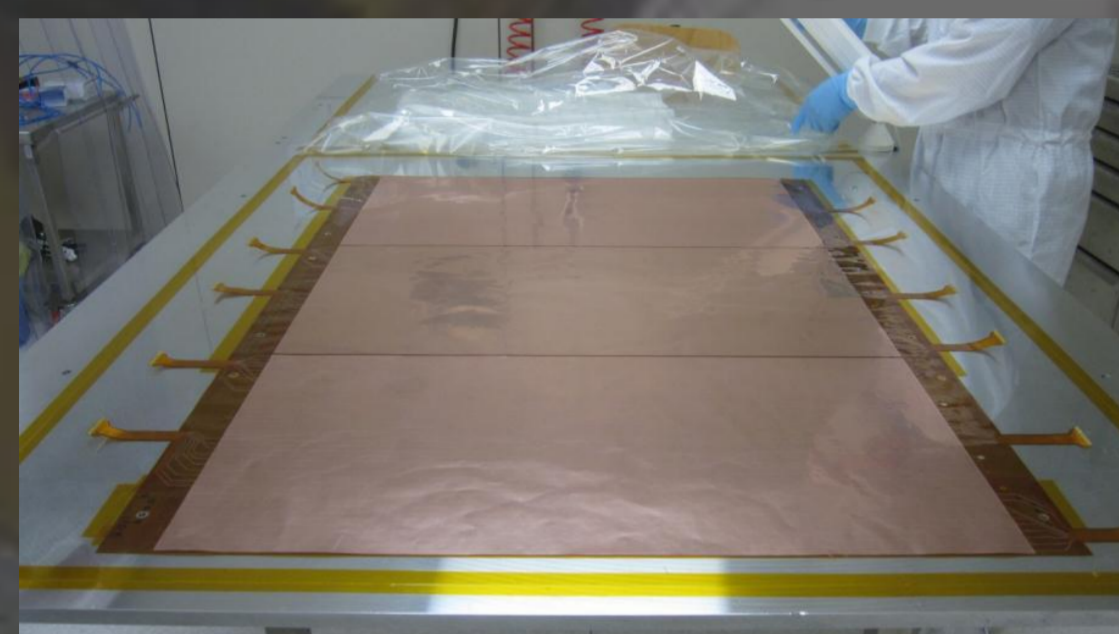
3 GEM foils are spliced together to obtain a 100x70 cm 2 electrode...
