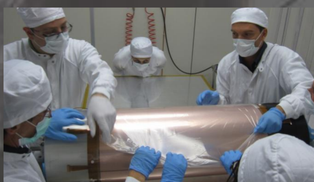
... that is rolled on a cylindrical mold and enveloped in a vacuum bag.
