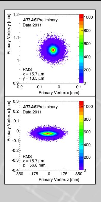
Vertex resolution is measured from data using the split-vertex method.
