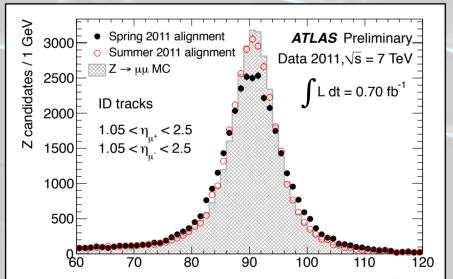
Resolution on track parameters is very near to expectation for the simulation of a perfectly aligned detector
