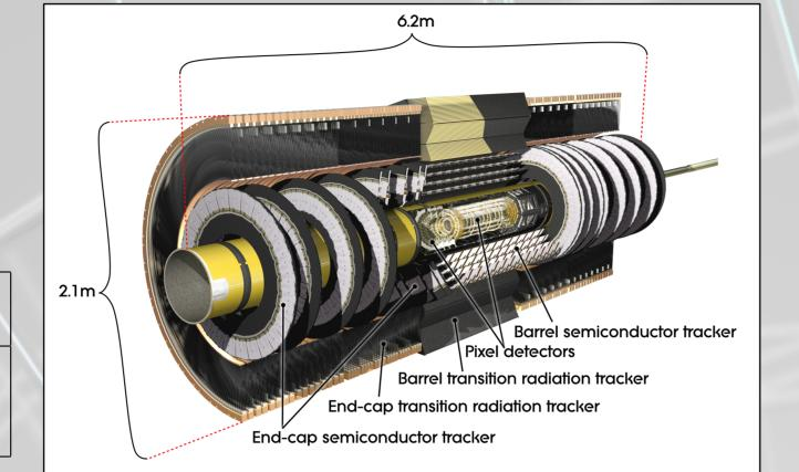
All these sub-detectors allow precision measurement of charged particle trajectories in the high-multiplicity LHC environment.
