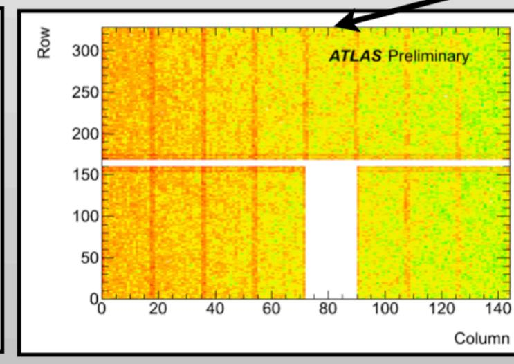
the lower efficiency for the most external disks is mainly due to inefficient regions on some modules
