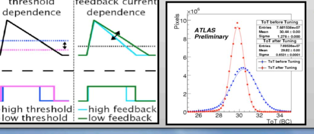
TOT tuned pixel by pixel to 30 BC @ 20 ke<sup>-</sup>
