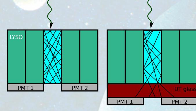
In order to promote light spread and avoid overlap of responses, ultra-transmitting (UT) glasses can be inserted between the crystal matrix and the PMT in order to gain pixel identification efficiency especially at the peripheral active area by exploiting the enhanced light spread.
