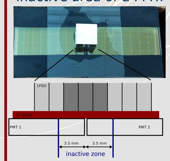
For our detector setup, the inactive area between two phototubes adds up to 7mm. With a crystal pixel pitch of 1.7 mm, four pixels are geometrically assigned to this region.
