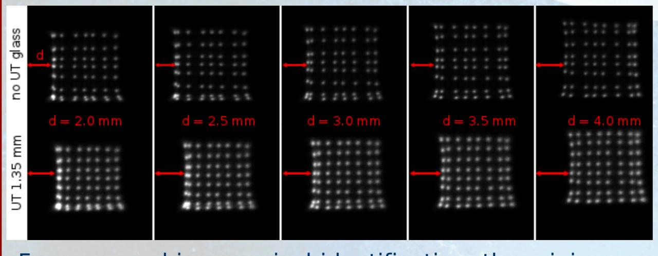
For an unambiguous pixel identification, the minimum distance to border is 3.5 mm for both setups, i.e. with and without UT glass.
