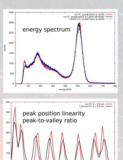
However, each pixel becomes slightly more diffuse with increasing glass thickness leading to a reduced peak-tovalley ratio and marginal the worsening of energy resolution. The following table summarizes the pixel identification properties.
