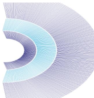
layout of  $R$  and  $\phi$  prototype sensors
