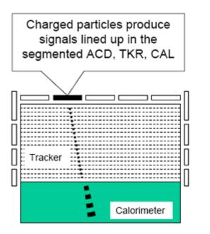
A high-energy gamma ray can produce secondary photons that "splash" out of the CAL and can trigger an ACD tile.
