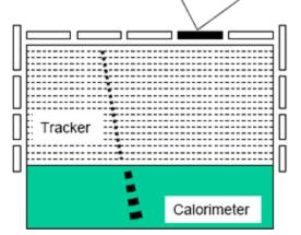
The ACD consists of an array of plastic scintillator tiles, which emit light when traversed by charged particles. By detecting these particles, the ACD helps identify and reject events caused by charged particles, allowing the LAT to focus on gamma-ray signals.
