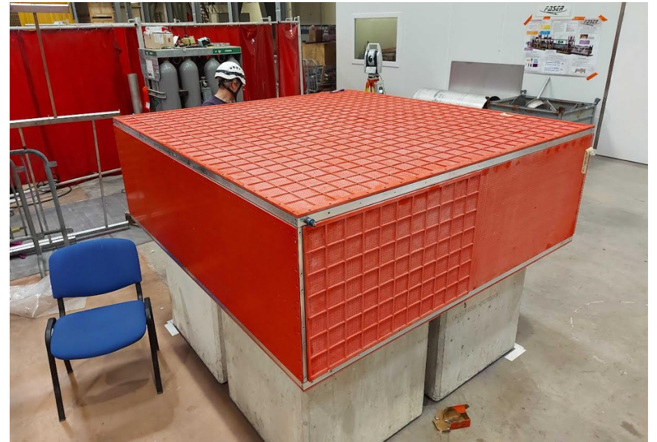
The Super-FGD box which carry all the cubes
