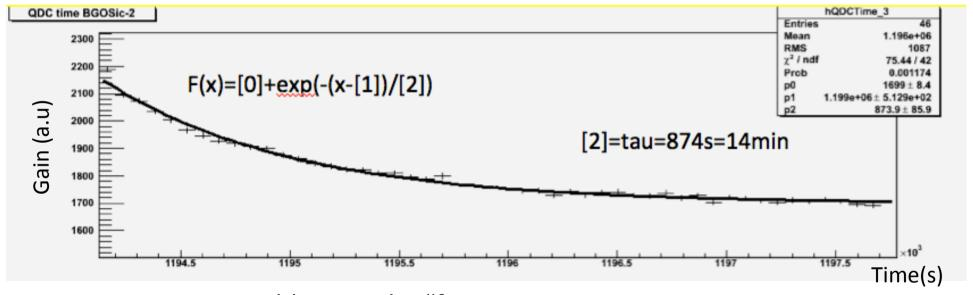
Impossible to make "fast measurements" with LY setup in irradiation zone
