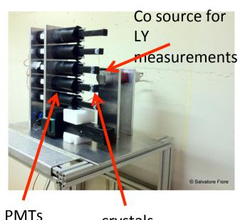
First measurement setup: crystals on PMTs during irradiation, HV ON during fast measurements between irradiations HV standby during irradiation
