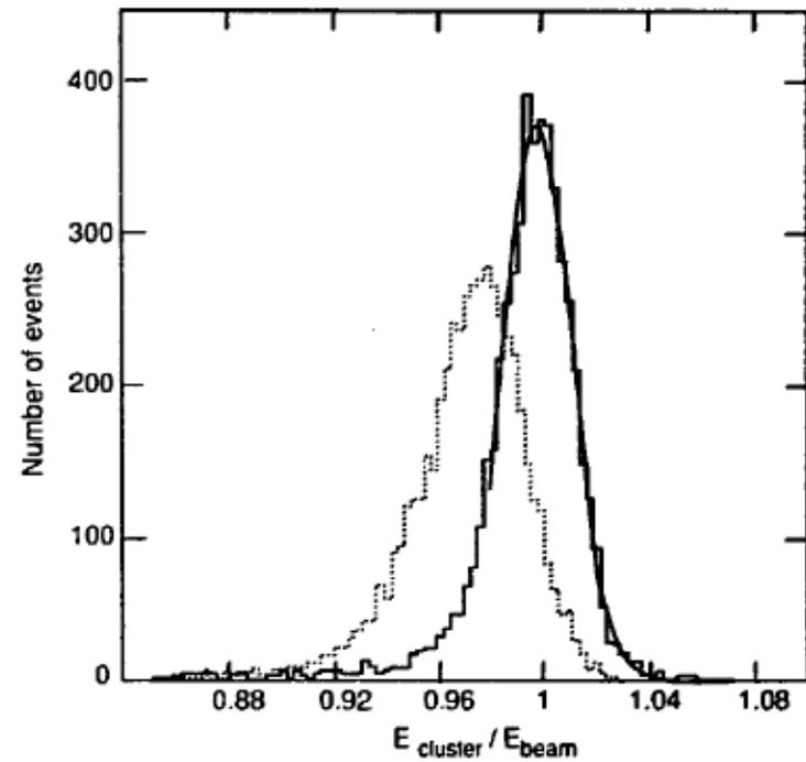
Fig. 15. Energy resolution of the BGO barrel. Dotted line: uncorrected data ( $\sigma^E = 1.70\%$ ). Continuous line: corrected data ( $\sigma^E = 1.25\%$ ).
