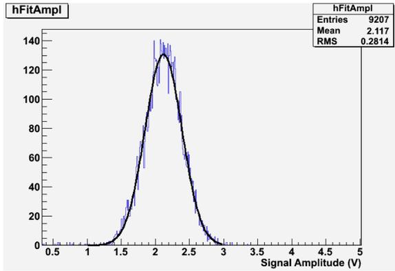
For each RC value between 20 ns and 500 ns we fitted the signal amplitude spectrum with a gaussian curve;
