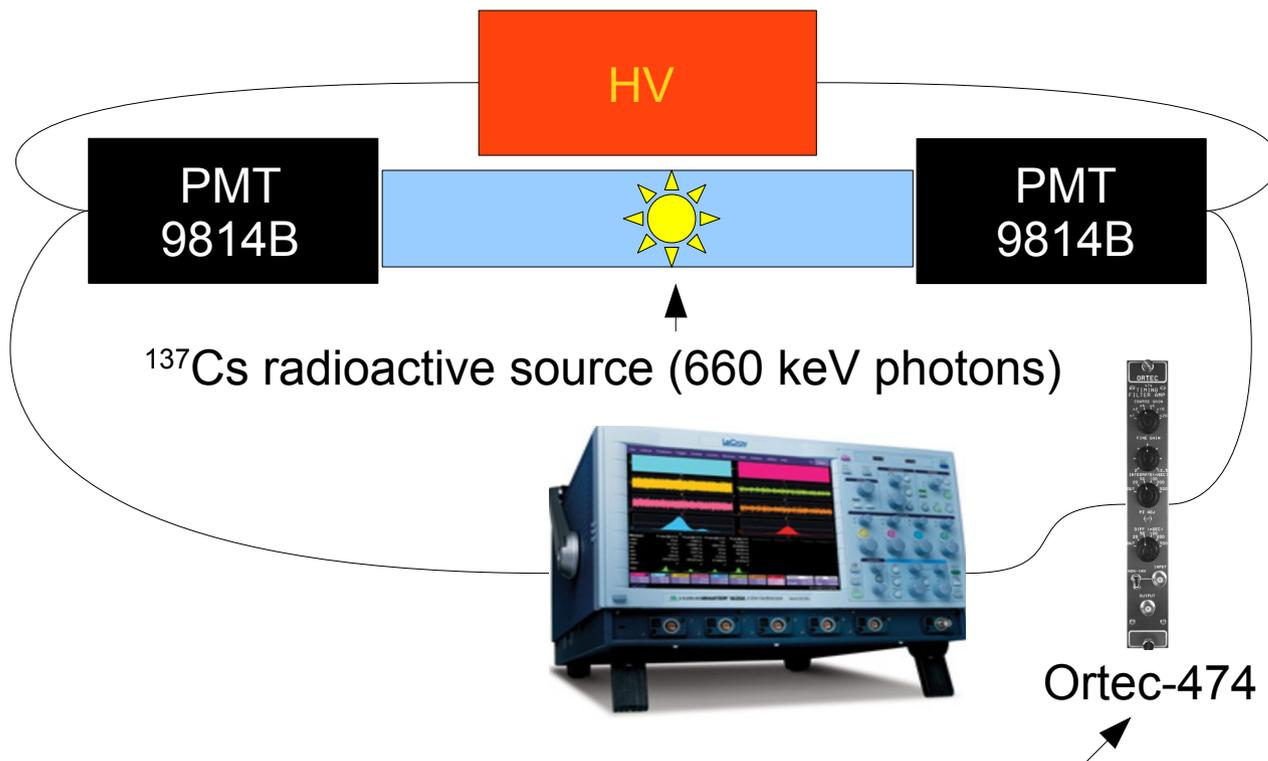
The energy resolution was studied as a function of the integration time of the readout for values of: 20ns, 100ns, 200ns and 500ns.
