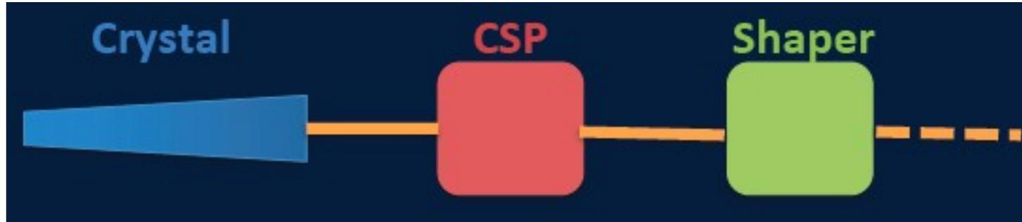
Since the Shaper part is linear, the statistical contribution to the energy resolution will be given by the fluctuations of  $A$ ;
