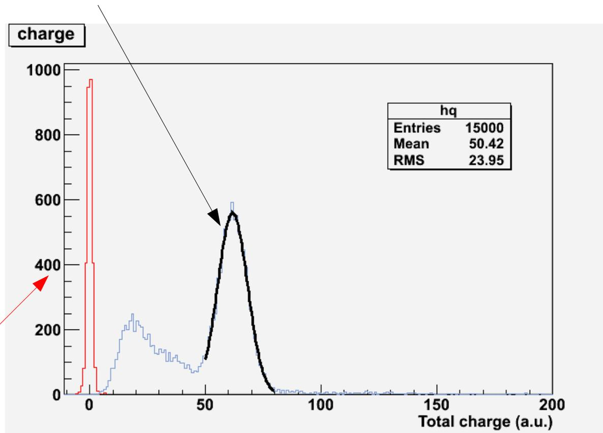
**Red:** charge spectra with the random triggers (i.e. the pedestal due to electronics noise). Its width is 10% of the signal peak width. Thus its contribution in quadrature is negligible.
