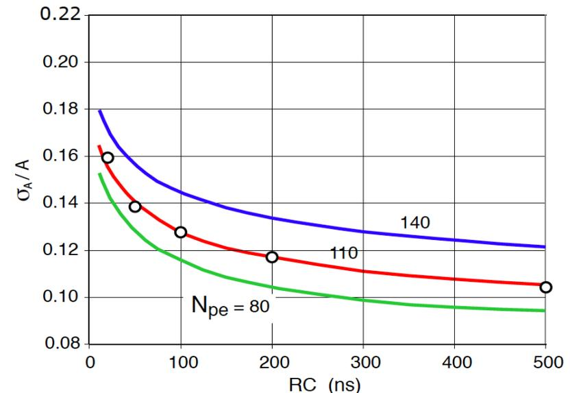
The results of the toy MC are compatible with the experimental data and seem to indicate a light yield of 110 p.e.
