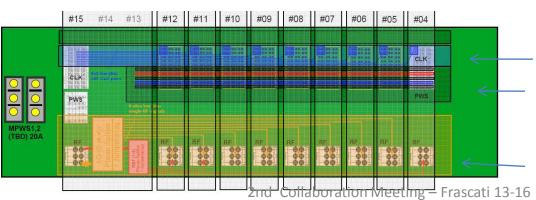
Low Jitter clock distribution < 200fs Independent redundant power supplies
