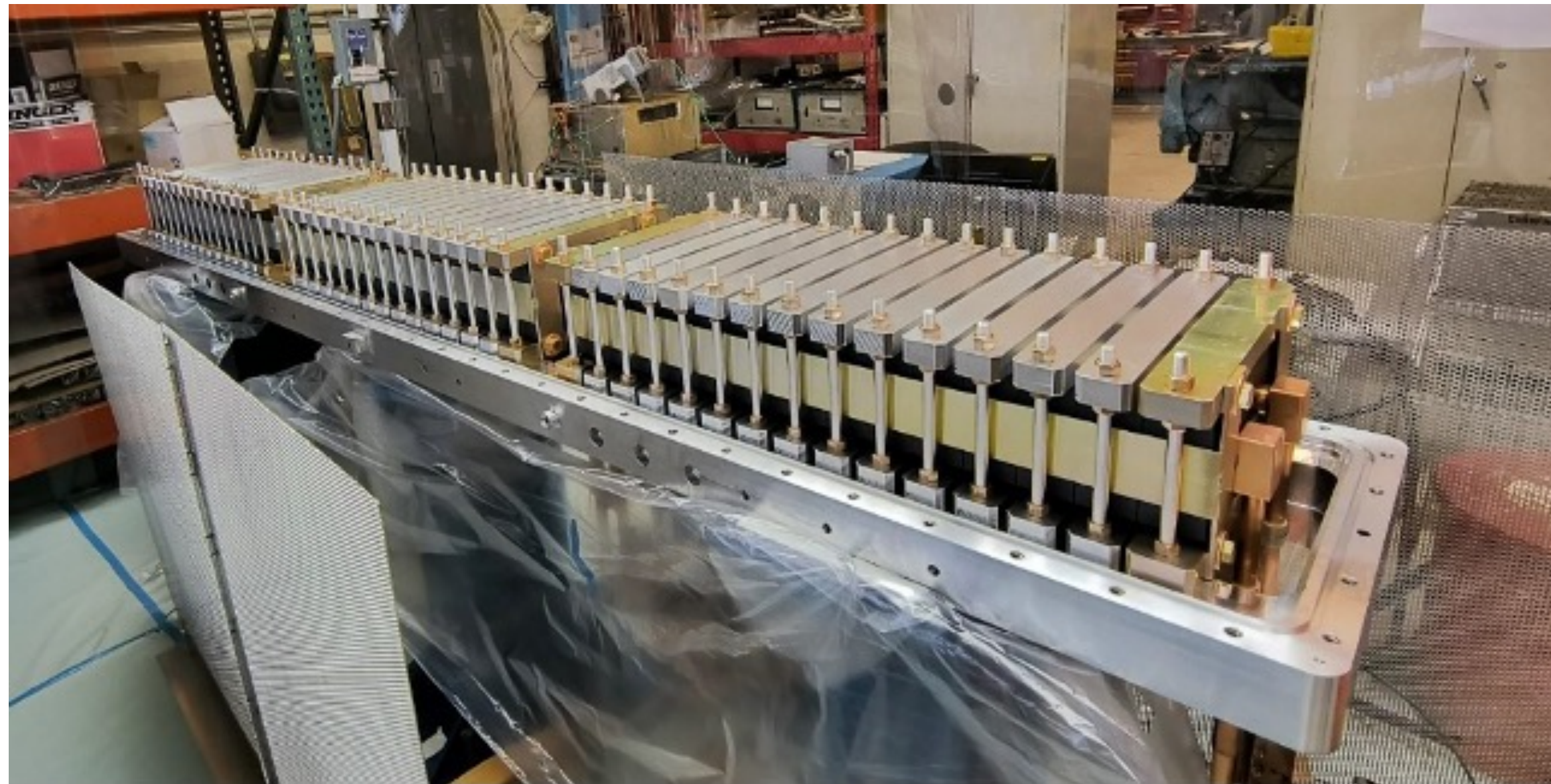
Built one AC dipole (pulsed beam), second one almost done, spare planned.
