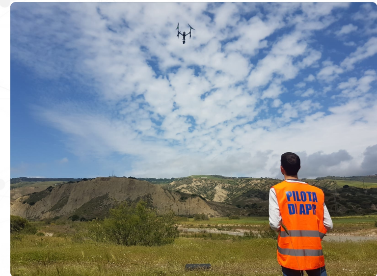
UAV survey using a DJI Inspire 2 equipped with DJI Zenmuse X5S optical sensor
