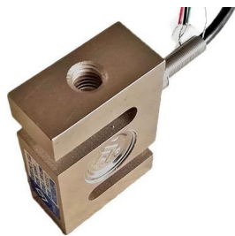
typical load-cell 24 (48) around perimeter
