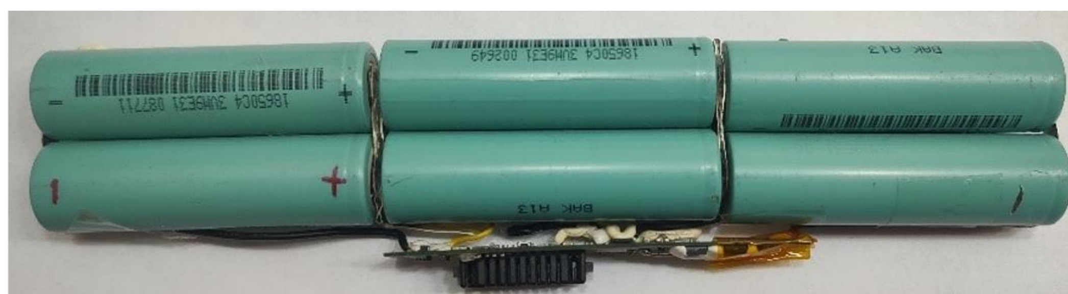
Fig. 2: Disassembled battery with the 18650 cells
