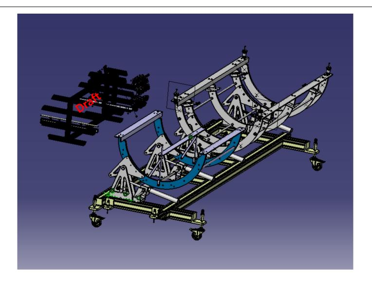
Mechanical structure for placing and supporting cables during the integration
