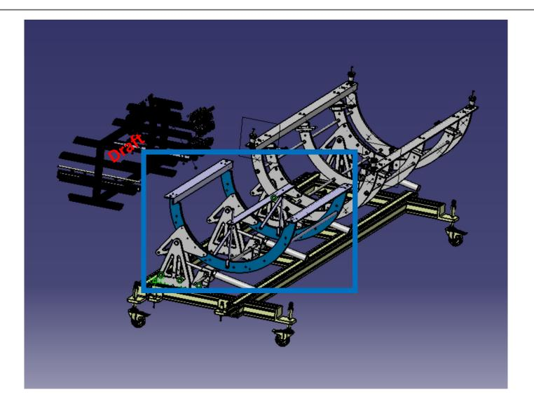
Mechanical structure for placing and supporting cables during the integration
