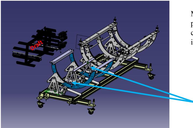
Mechanical structure for placing and supporting cables during the integration
