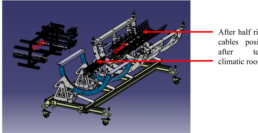
After half rings and cables positioning, tests in climatic room
