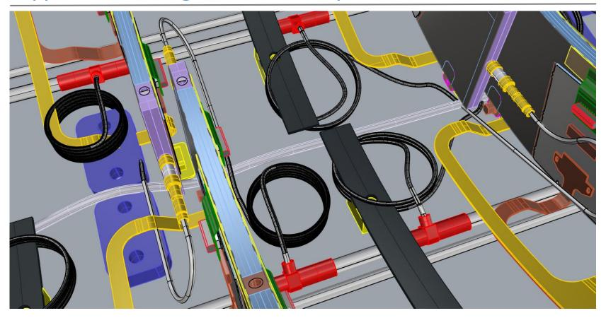
Identified & discussed at Edinburgh but no time to fix due to preparations for FDR. Plan is to investigate turning capillary coils through 90 degrees – might also help with clashes during HC joining.
