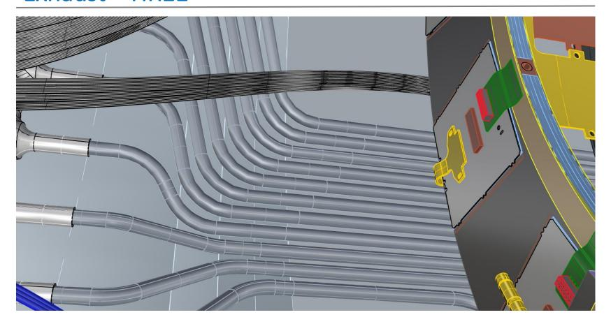
I have a DataPPO here – I do not believe the bends assumed in the 3D modelling are realistic – unless there is a 'feature' on the outer rim of the half-ring to fix the DataPPO finger to. Suggest moving group of 4 exhaust tubes round in phi.
