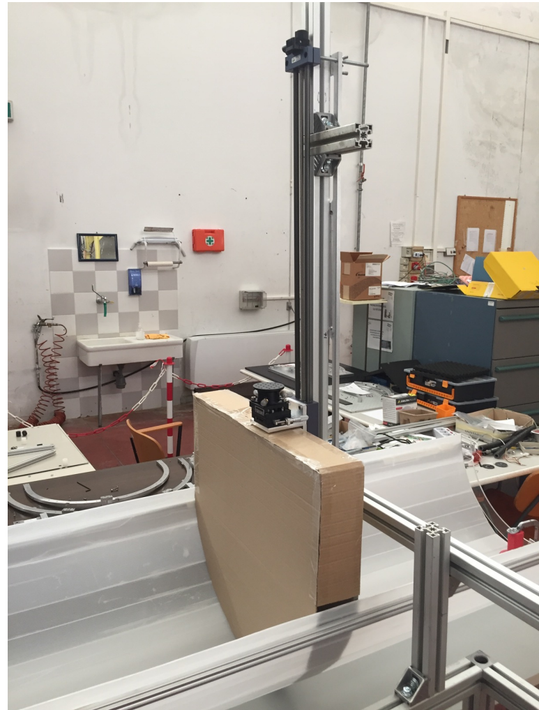
Half-ring testing enclosure mock-up
