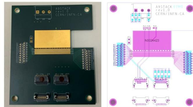
*the first prototype of the A9 stack carrier board.*
