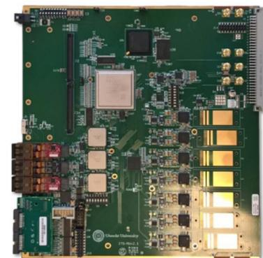
*Fig. 8 - Readout Unit to be employed for the A9 stack*
