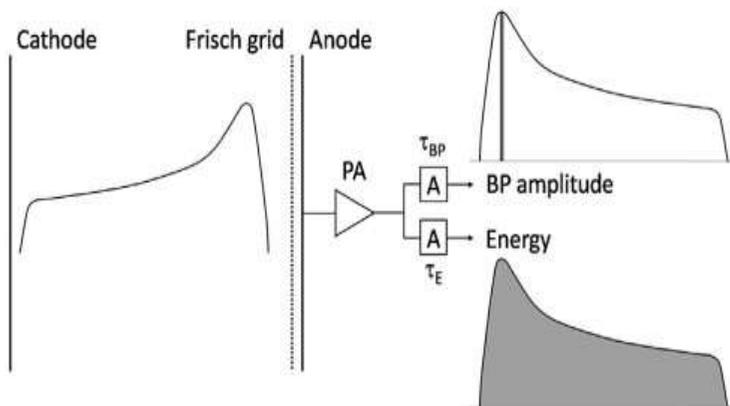
illustration of the Bragg Curve Spectroscopy principle
