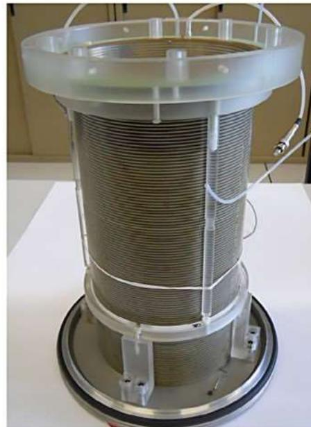
inner structure of the Bragg chamber
