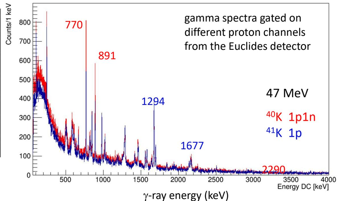
gamma spectra gated on different proton channels from the Euclides detector
