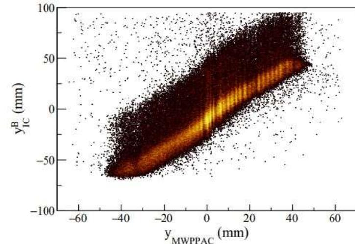
A matrix of  $Y_{\text{MWPPAC}}$  vs  $Y_{\text{IC}}$  has been constructed, showing a quite good linearity and demonstrating the good planarity of the ion trajectories at the focal plane
