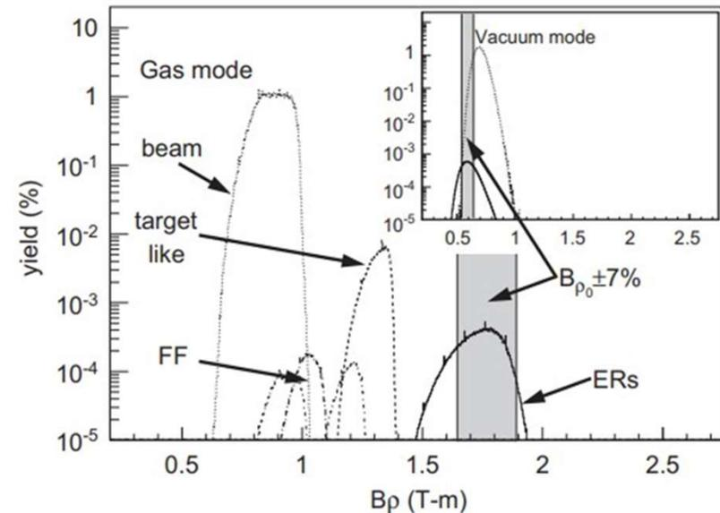
calculated magnetic rigidities of the reaction products with the spectrometer filled with He gas at  $p=0.6$  mbar
