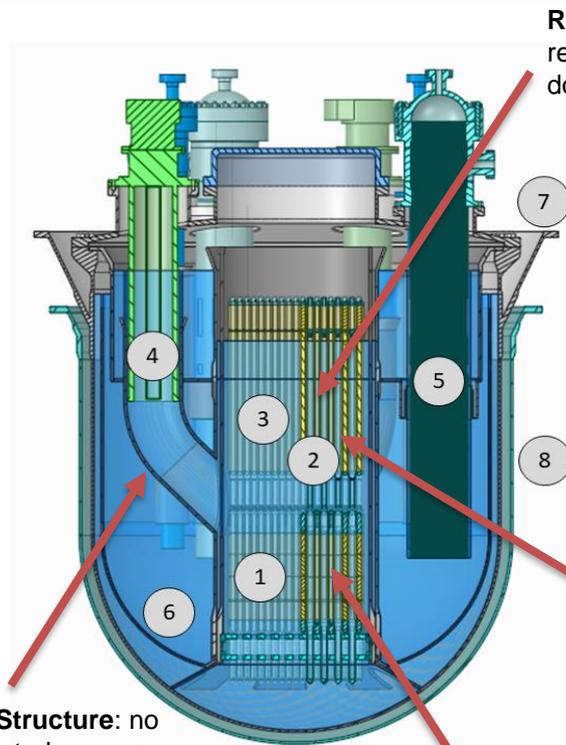
**Reactivity control:** Two diverse and redundant systems, control and shut-down rods
