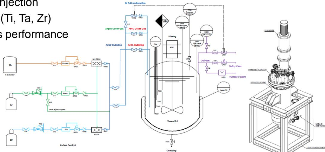
HLM mixer to study the effect of fluid-dynamic conditions on oxygen control
