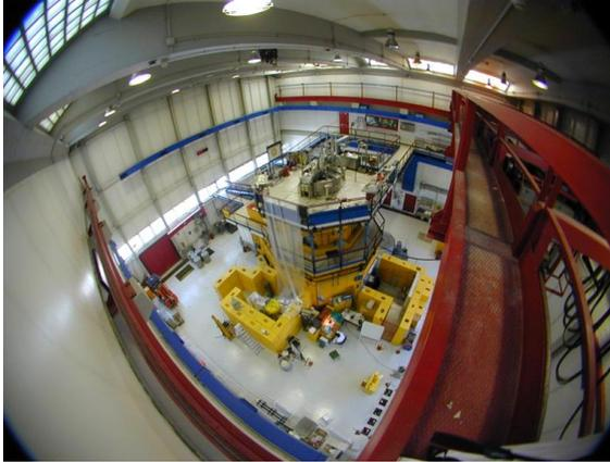
**TRIGA RC-1:** 1 MW power,  $2.7 \cdot 10^{13}$  n cm<sup>-2</sup> s<sup>-1</sup> thermal neutron flux nuclear research reactor
