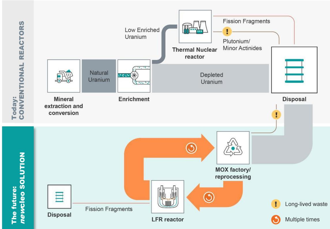
Thermal fission reactors use a very small portion of the extracted uranium: an average 1GWe LWR uses every year 200t of mined uranium of which only 1t is fissioned (Fission Products), the rest is “waste”
