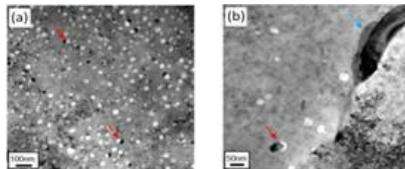
Low amount of cavities in the advanced austenitic stainless steel (b) if compared to the non-optimized 15-15 Ti (a)
