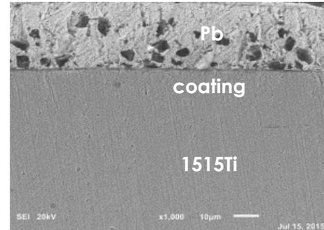
1  $\mu\text{m}$   $\text{Al}_2\text{O}_3$  coating
