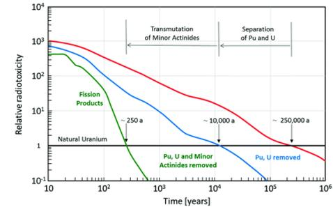
Fast Reactors and fuel reprocessing can extract energy from existing material and at the same time reduce radiotoxicity of residual waste to dispose: Fission Products return to value of the natural uranium ores after ~250 years
