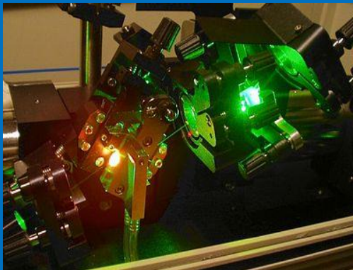
Ti:Sa laser Pumped with laser light
