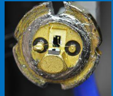
DIODE Laser: electronic current pump
