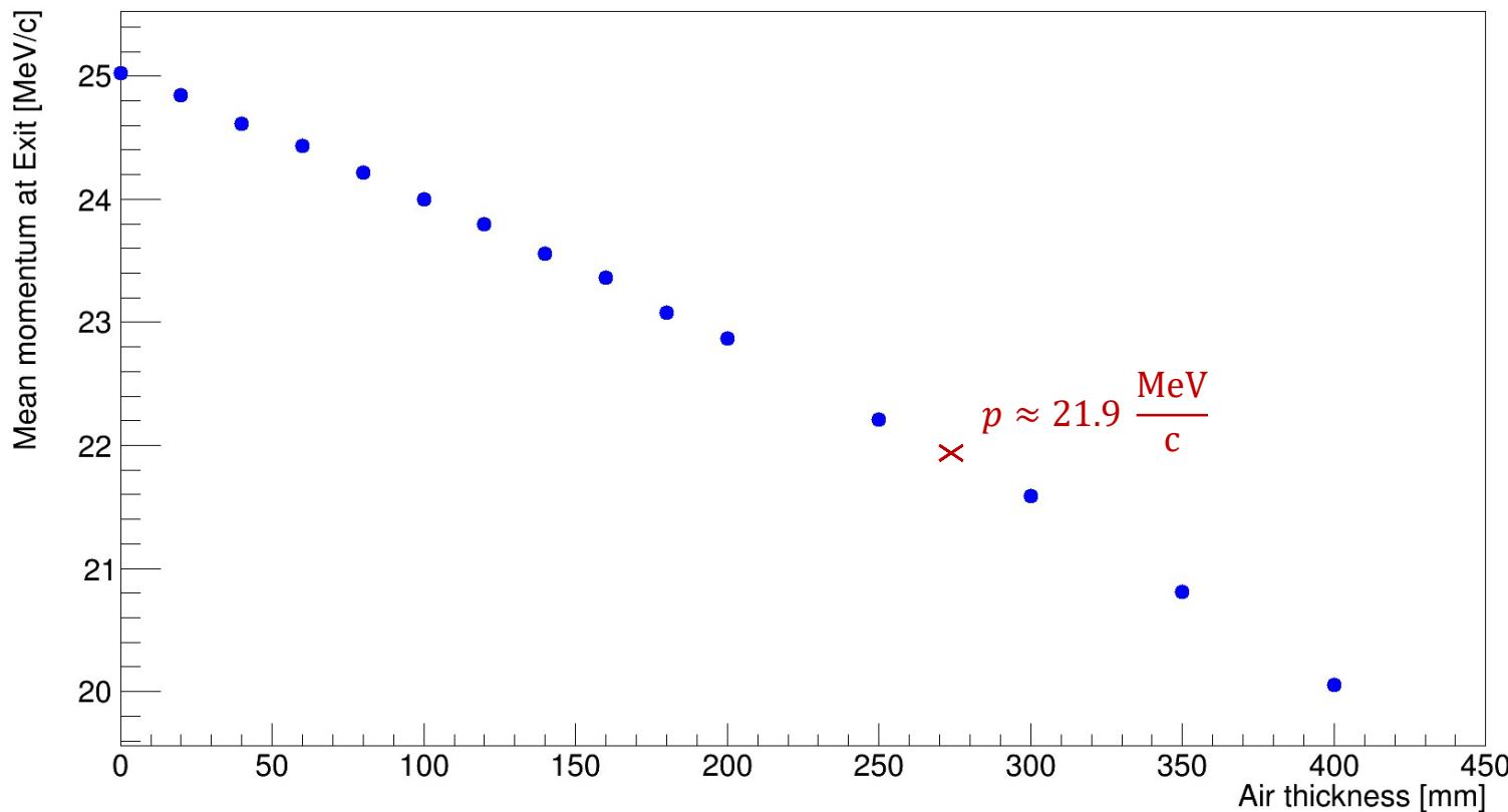
Mean muon momentum after exit scintillator depending on the air thickness, simulated in G4Beamline
