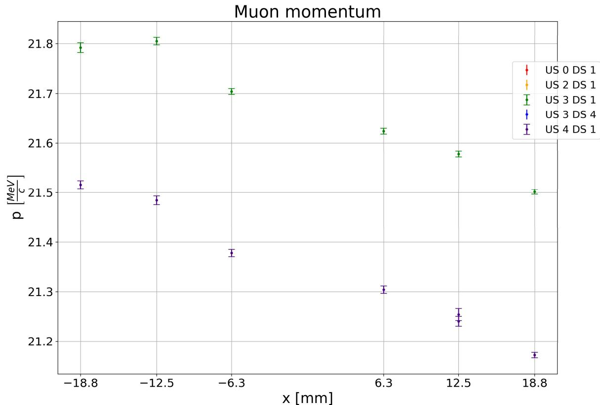
Mean muon momentum when changing the position of the magnet
