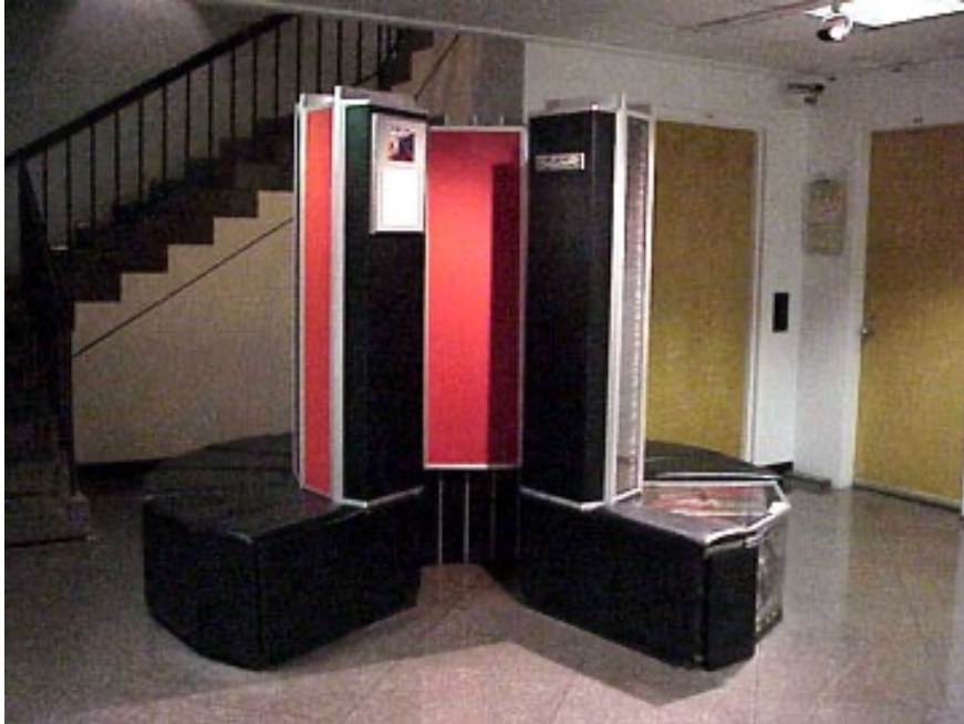
Cray 1, 1977, first real supercomputer, 110 MFLOPS (Linpack 1000)
