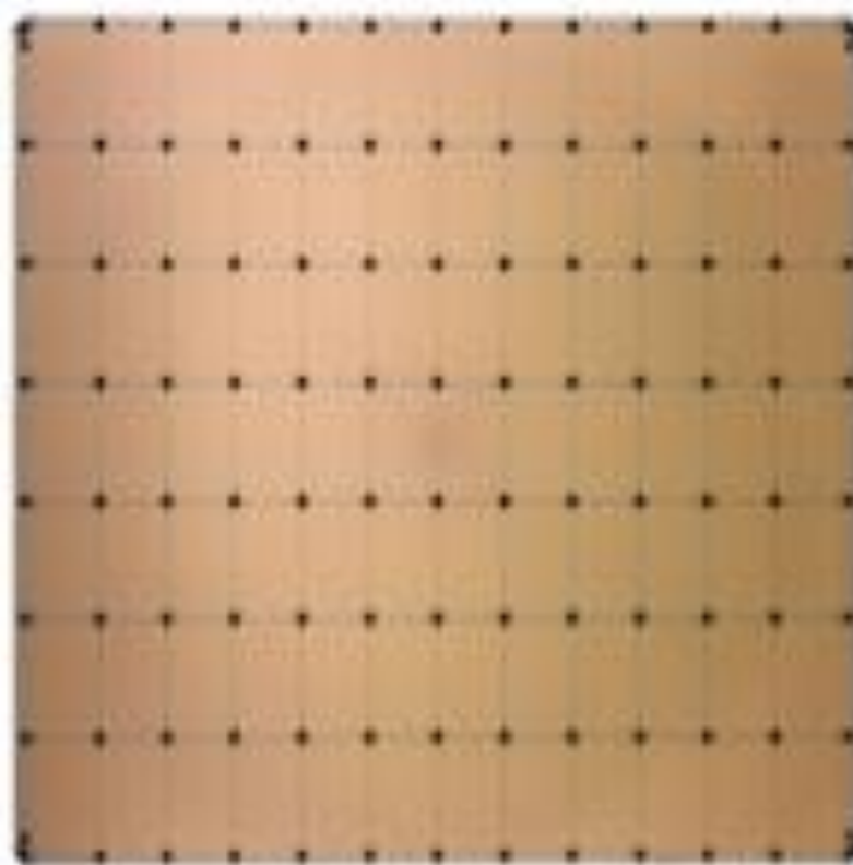
Cerebras WSE-3 4 Trillion Transistors 46,225 mm 2 Silicon
