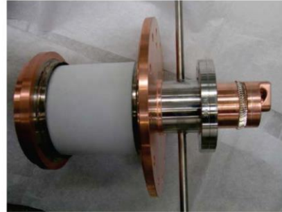
Figure 1: RF coupler system with loop, coaxial transmission line and coaxial alumina window.
