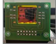
Charge selective contact detector on glass substrate
