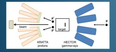
coincidence measurement of gamma rays and scattered protons
