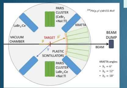
KRATTA inside the **chamber** – in the vacuum gamma detectors outside mounted using holders / cylindrical pockets
