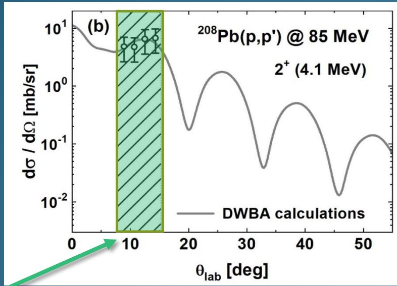
the angles covered by the experimental setup
