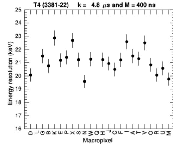
Energy Resolutions close to specifications for alpha particles (< 20 keV FWHM)
