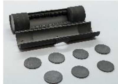
SPES SiC target (1600°C)
