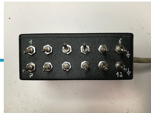
Filtering and grounding box
