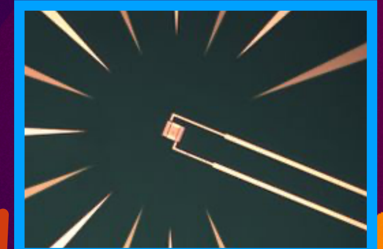
Tungsten microchip operating at T_C \sim 140 mK. from NIST ( 25 \mu\text{m} \times 25 \mu\text{m} \times 20\text{nm} )
