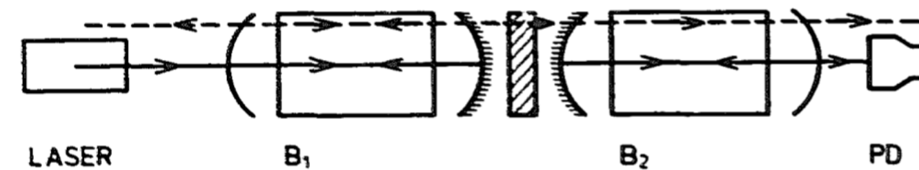
Fig. 3. Axion production and detection with two optical resonators.
