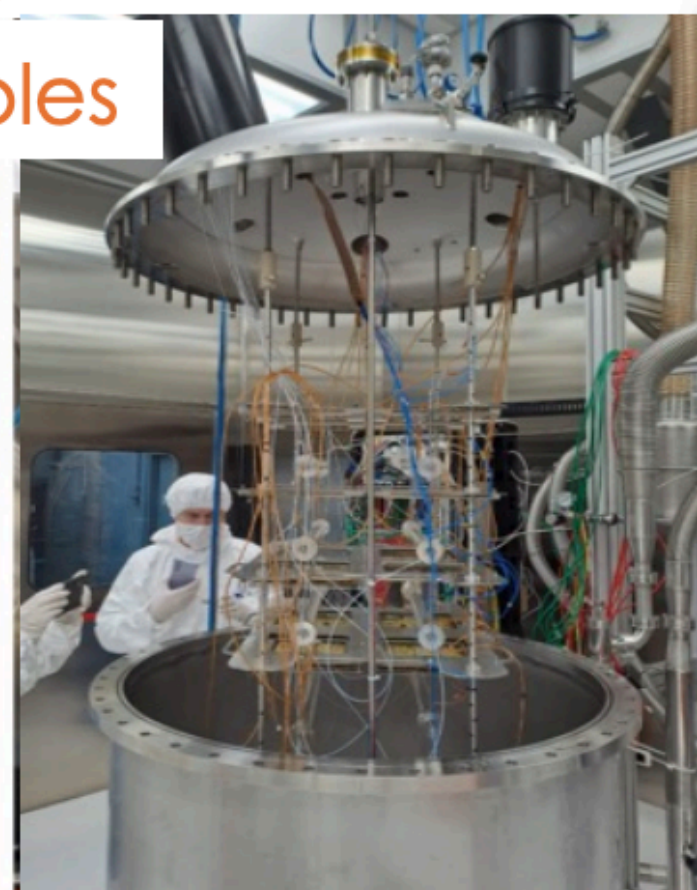
Assembly PDUs will be tested in a cryogenic test facility in Naples – vPDUs will be tested in facilities at AstroCeNT, Edinburgh and Liverpool
