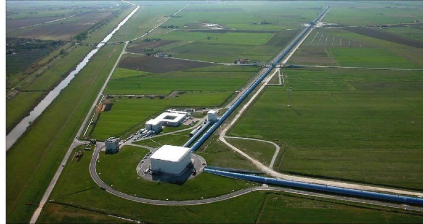
Aerial view of the Virgo interferometer operated by CNRS and INFN (Cascina, near Pisa, Italy). European Gravitational Observatory (EGO) is an European consortium which controls Virgo. The arms length is 3 km.
