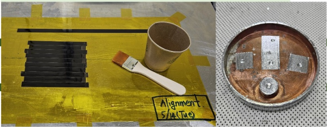
HTS preparation & Lid masking with Al tapes
