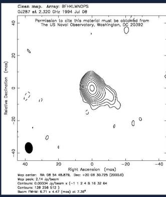
The dark image on the left side of the picture is the antenna diagram, which shows at what distances 2 different sources can be separated from each other.
