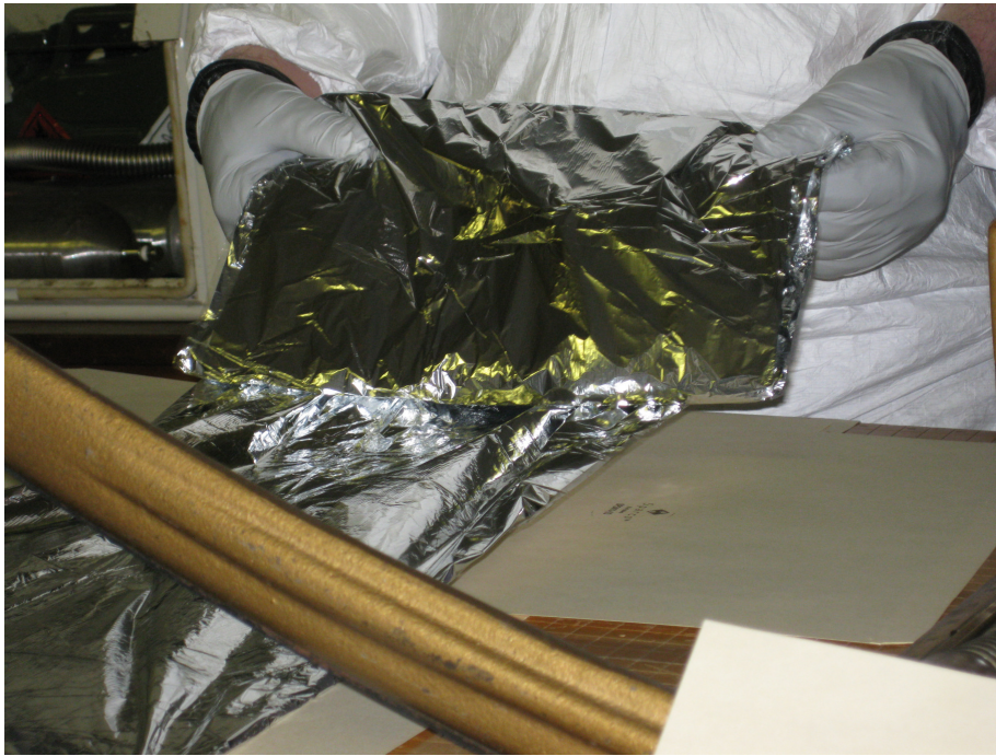
Figure 8: While Eric pulls on the far end of the film, Daniel feeds the film off of the roll and applies tension from his end. Shown above is a folded package of practice 2\mu\text{m} thin-film rather than the proper roll one would see from the final-product material.
