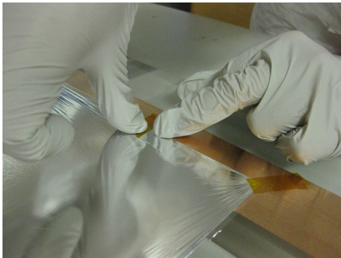
Figure 13: Daniel finishes the application of a piece of kapton tape by pressing down firmly on it.
