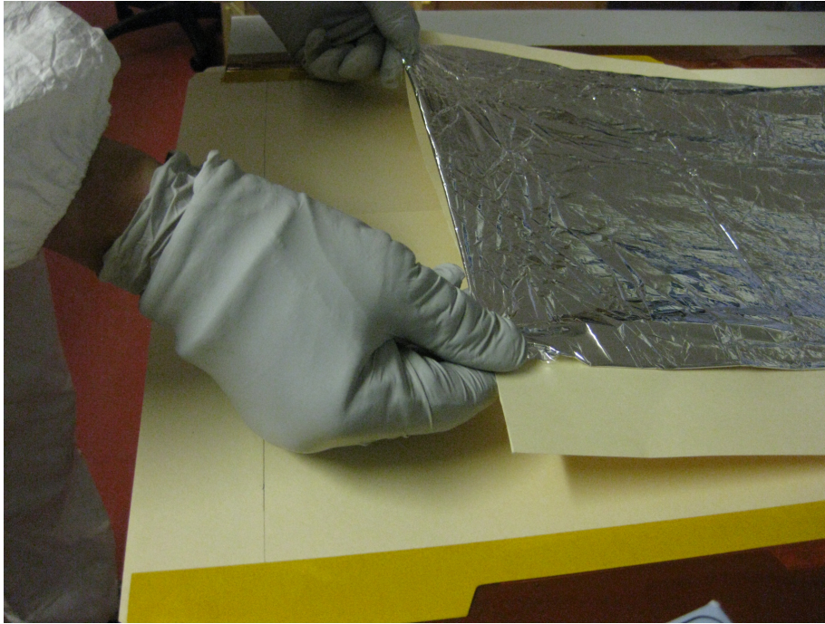
Figure 7: Eric pulls the thin film until it is aligned with the proper-length measurement drawn earlier. He also ensures the film is perpendicular to the cutting edge of the paper-cutter.
