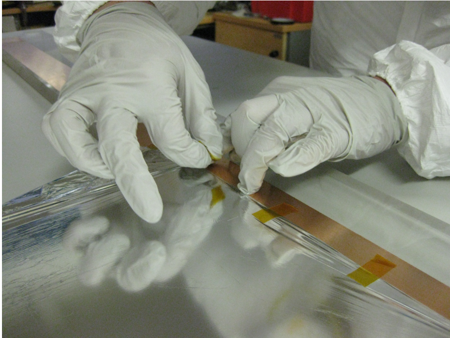
Figure 17: The two stretchers work together to lay down piece of kapton tape (with release tabs), starting from the aligned edge and moving toward the free edge.
