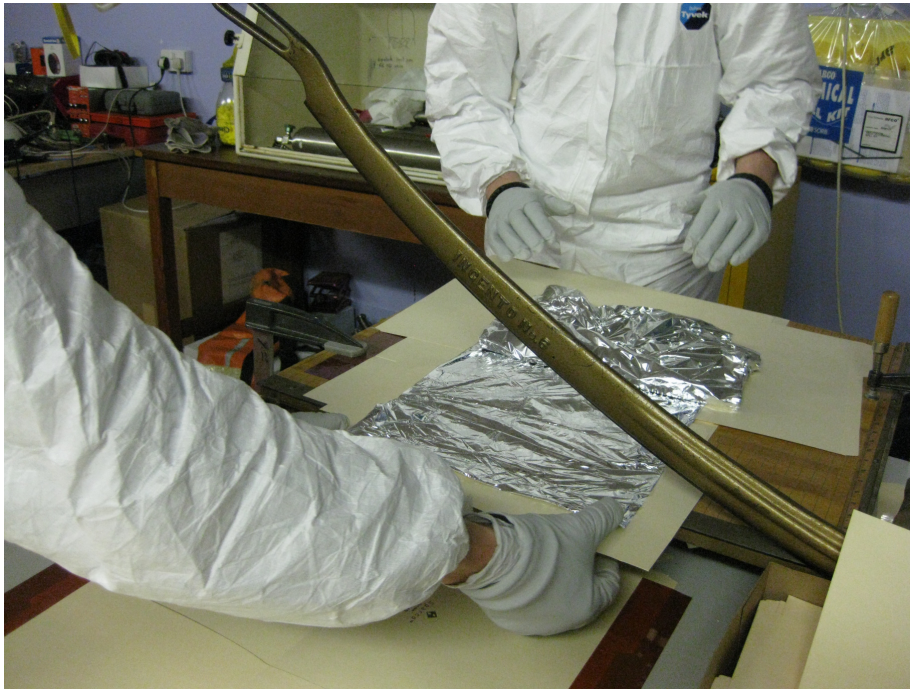
Figure 6: Daniel Walker has pushed the thin-film on its manila base past the cutting plane of the paper-cutter, allowing Eric Lee to grab ahold of it and pull without passing his hands through the cutting plane.
