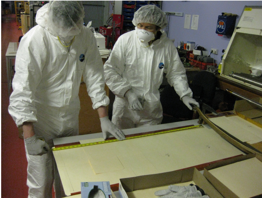
Figure 5: Eric Lee and Daniel Walker finish preparing a work area for cutting the thin-film. Here the paper-cutter is secured with wood clamps and the layout surface for the film (including the top of the paper-cutter) is covered with manila folder. Eric and Dan are performing the final measurement to mark the length of one full panel from the cutting line. The blade of the paper cutter is kept closed and secured whenever possible.
