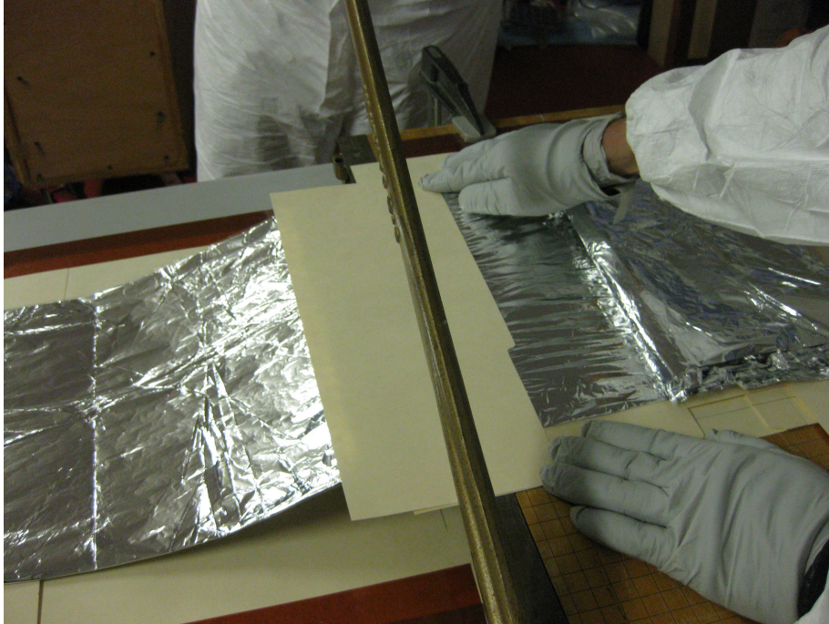
Figure 10: When the film has been rolled out to the appropriate length, a second piece of manila is placed above the film, completing the manila sandwich. Here the sandwich is secured for cutting by pressing down on the edges so as not to damage the film.
