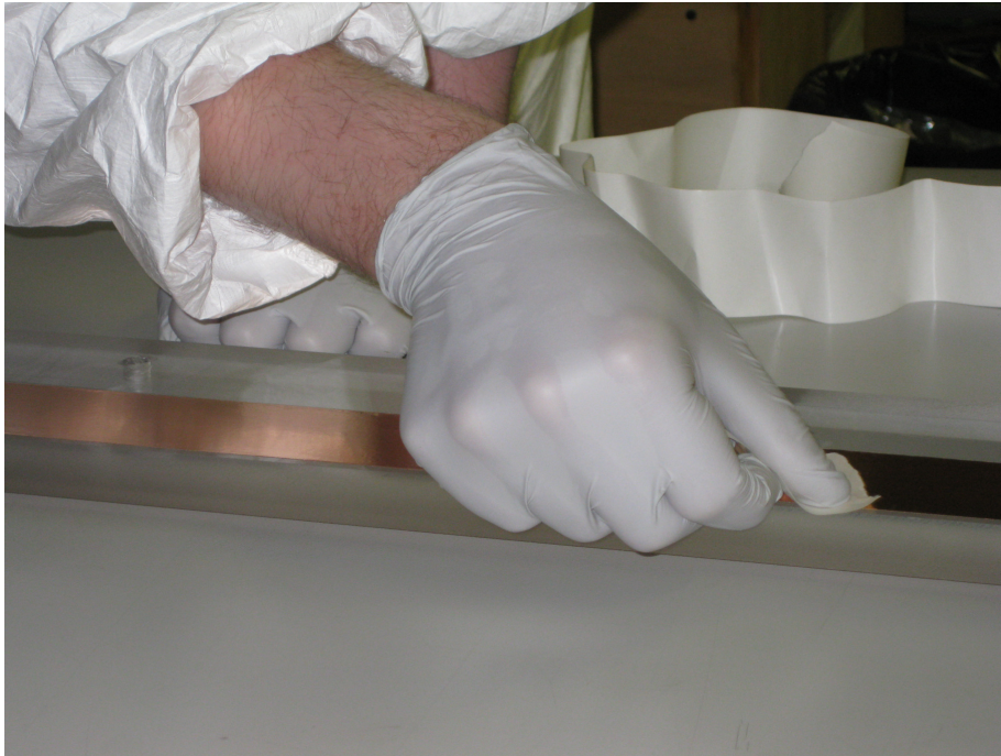
Figure 4: Daniel smooths down the copper tape with a piece of the wax backing paper.
