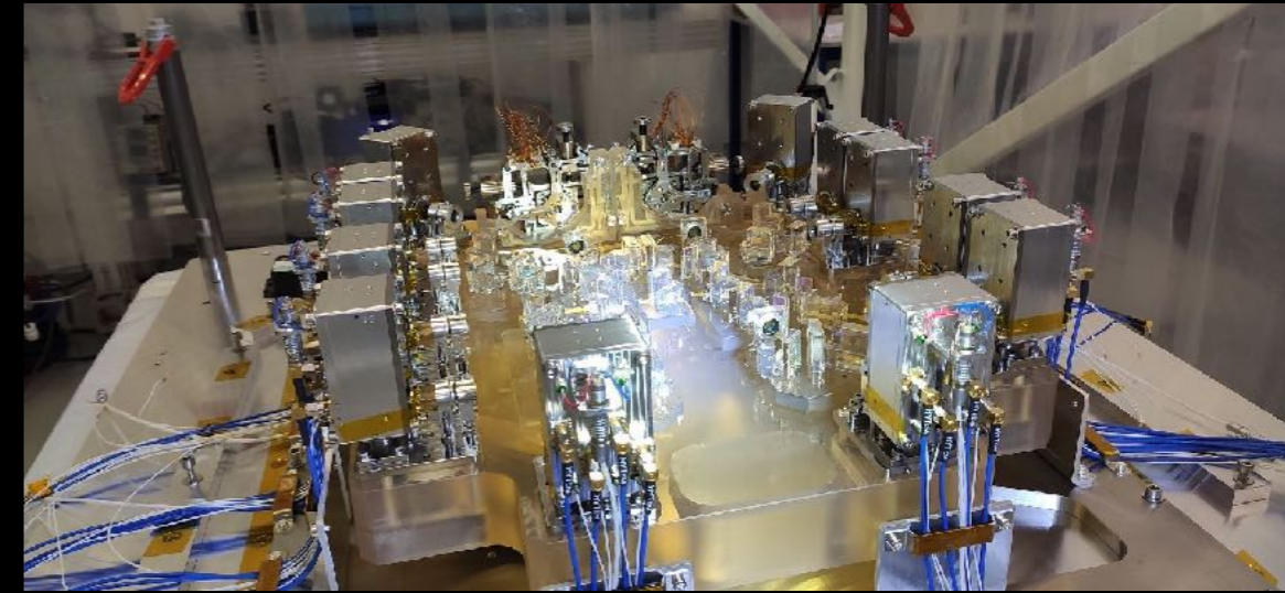
ZIFO (demonstration bench for high stability interferometry)
