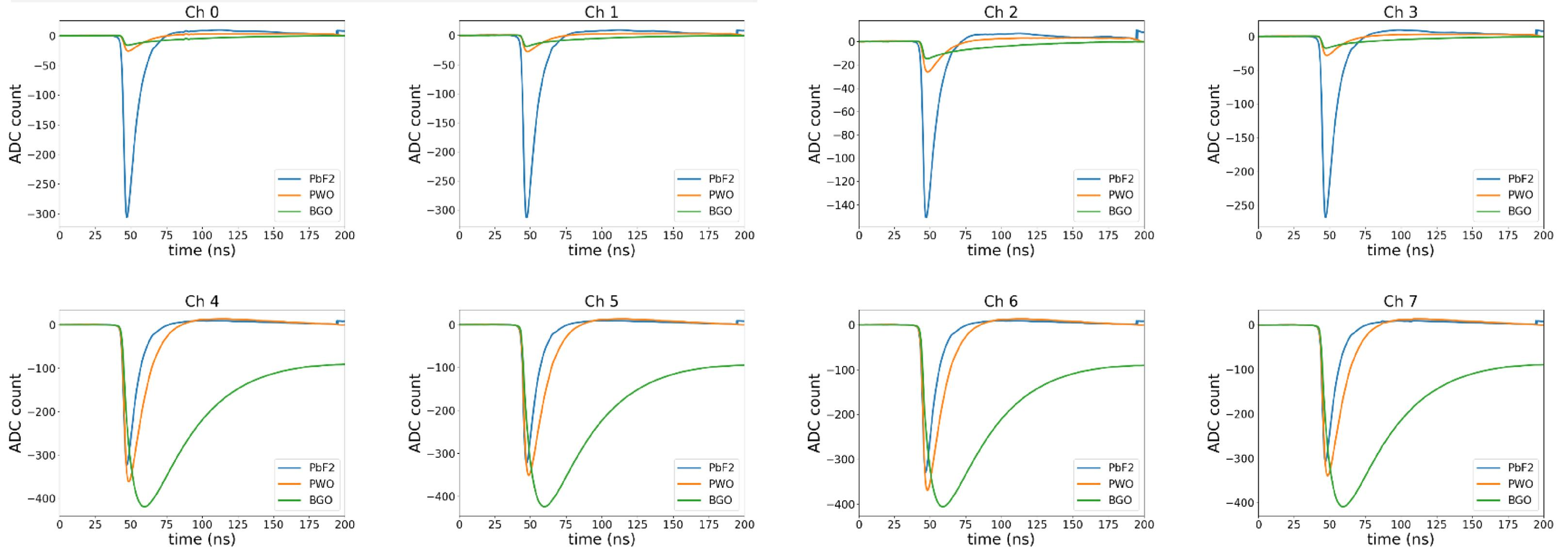
CH4-7 w/o filters for PWO & BGO: Different tail shapes due to scintillation decay time
