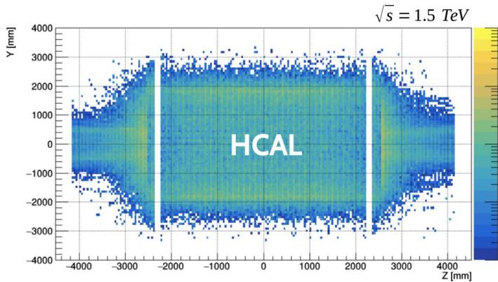
density of BIB hits vs calorimeter barrel depth
